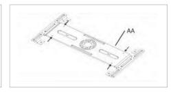
Using the mounting plate as a guide, mark the position of the holes in the ceiling or wall where the toggle bolts will be placed
