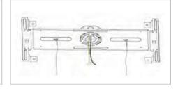
Hook the support wire from the fixture on the mounting bracket plate
