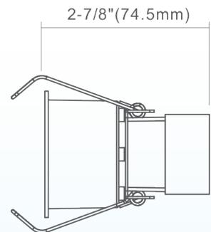
Ceiling Cut-Out Hole Size: Ø2"
