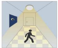
With insufficient daylight, when motion detected, light ON.
