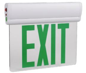
Now available is the EnVision Edge-Lit LED Emergency Exit Sign. Available in a green and red light, with a single sided and double sided version, place these signs on walls or ceilings near exit locations. With a nickel cadmium battery, the charging time for this fixture is 24 hours, with a discharge time or backup time of 90 minutes. Make sure everything works correctly with a test switch and charge indicator.
