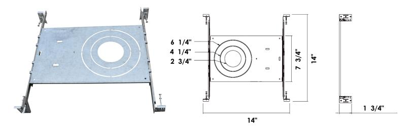
The EnVision LED Universal Mounting Plate, is a new construction pre-mounting plate with a collar for use with screw down "C" style remodel housings.
