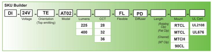
Example: **DI-24V-TE-AT02-400-32-FL-PD-8'2"-RTCL-UL2108** = Diode, 24 Volt, Top emitting, AlphaTECH® 400 Type 2, 400 Lumens, 3200 CCT, Flexible, Premium Diffused, 8 feet 2 inches, 96" lead, with rotating mounting clip, and UL2108 Certified.
