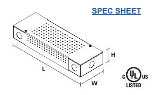
**LO-PRO**<sup>®</sup> JUNCTION BOX & DRIVER COMBO - 24V COMMERCIAL GRADE 0-10V LED DIMMABLE DRIVER Compatible with 0-10V controls and dimming systems.
