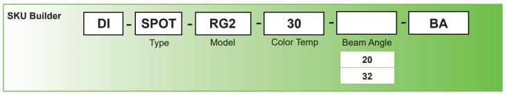
Example: DI-SPOT-RG2-30-20-BA = Diode LED, SPOTMOD 2 Recessed Gimbal, 3,000K CCT, 20 degree beam angle.
