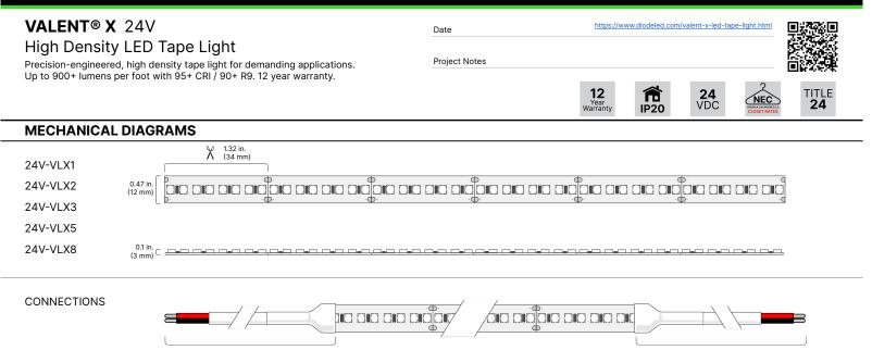
36 in. Bare Lead 20/2 AWG UL 2464 Wire with Strain Relief
