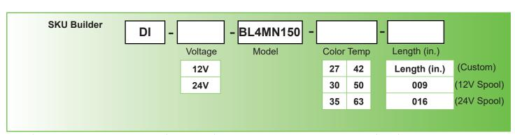
Example: DI-12V-BL4MN150-27-016 = Diode LED, 12 Volt, BLAZE™ MINI 150 4mm, 2,700° CCT, 16.4' spool.
