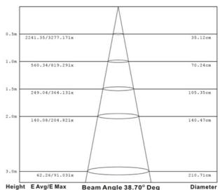
Beam Angle 38.70° Deg Note: The curves indicate the illuminated area and the average illumination when the luminaire is at different distance.
