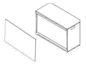
3. Pour the media into the tray. Feel free to use any combination of the fire glass media that you find most appealing. Insert the front glass panel back in place after the media installation has been completed.
