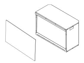
3. Unscrew the 2 screws located on each side and take off the inner side steel panels.
