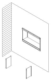
7. Insert the front glass panel back in place after the media installation has been completed.
