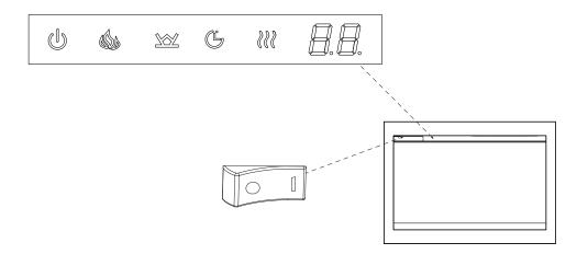
Touch the control panel once to "wakes up" the controls. This will cause the controls to light up. At this time, you can press the power button to turn on fireplace
