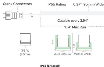
Features a clear protective silicone jacketing that protects the tape light from spraved water and dust. Best suited: Indoor & Outdoor damp & wet locations
