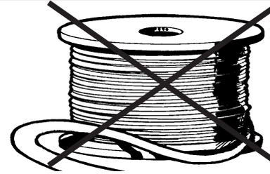
*Do not operate Polar 2 Mini Neon while it is coiled on the reel.*
