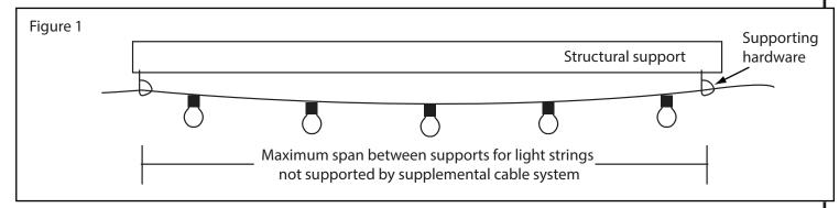
3. For spans exceeding the above, use properly rated cable support system and cable ties (both not provided) and follow local codes for suspended structures and loads.
