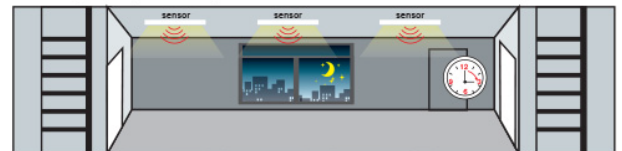
After standby period of no motion, fixtures return to desired dimming level (10%-50%).
