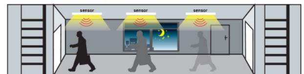
After standby period of no motion, fixtures return to desired dimming level (10%-50%).
